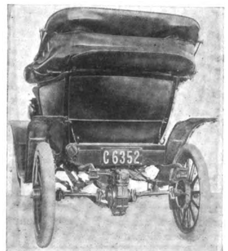
Showing Position of Power Plant.
